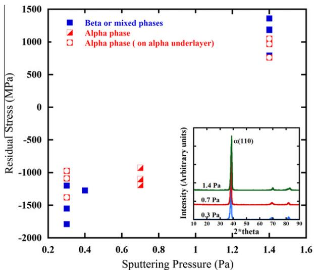
**Figure 4.** Plot of the residual stress of  $\alpha$ -Ta deposited at different sputtering pressures (0.3, 0.7 and 1.4 Pa) using an  $\alpha$ -Ta underlayer. Data points from Figure 2 are shown for reference (full square symbols). Note the formation of  $\alpha$ -Ta at all three different sputtering pressures. Inset presents the XRD spectra of the films processed at 0.3, 0.7 and 1.4 Pa, respectively, using an  $\alpha$ -Ta underlayer.
