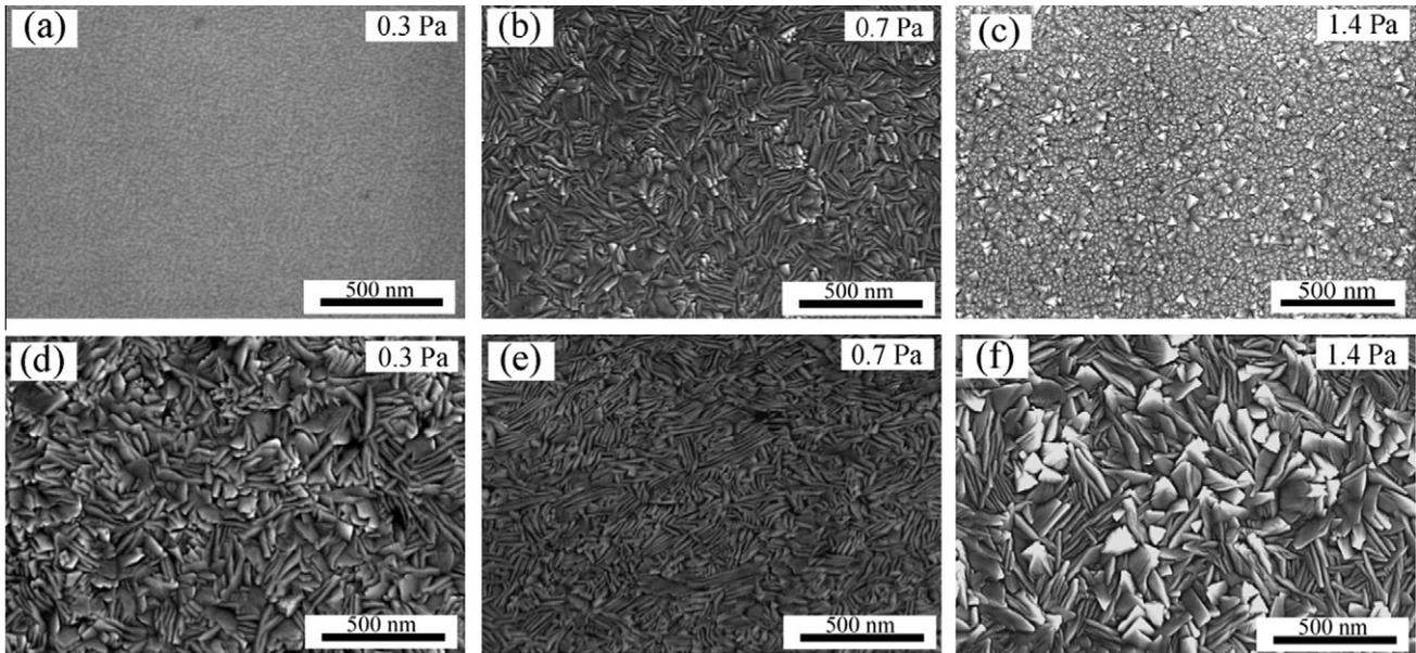
**Figure 3.** SEM images of the surface morphology of Ta samples synthesized at 100 W using three different sputtering pressures, 0.3, 0.7 and 1.4 Pa, deposited on two types of substrate surfaces: (a)–(c) Si substrate surface; (d)–(f) an  $\alpha$ -Ta underlayer surface.
