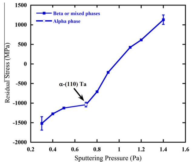
Figure 2. Plot of the residual stress as a function of sputtering pressures from 0.3 to 1.4 Pa. Arrow denotes  $\alpha$  phase at 0.7 Pa. All other pressures have a pure  $\beta$  or a mixture of  $\alpha$  and  $\beta$  structures.
