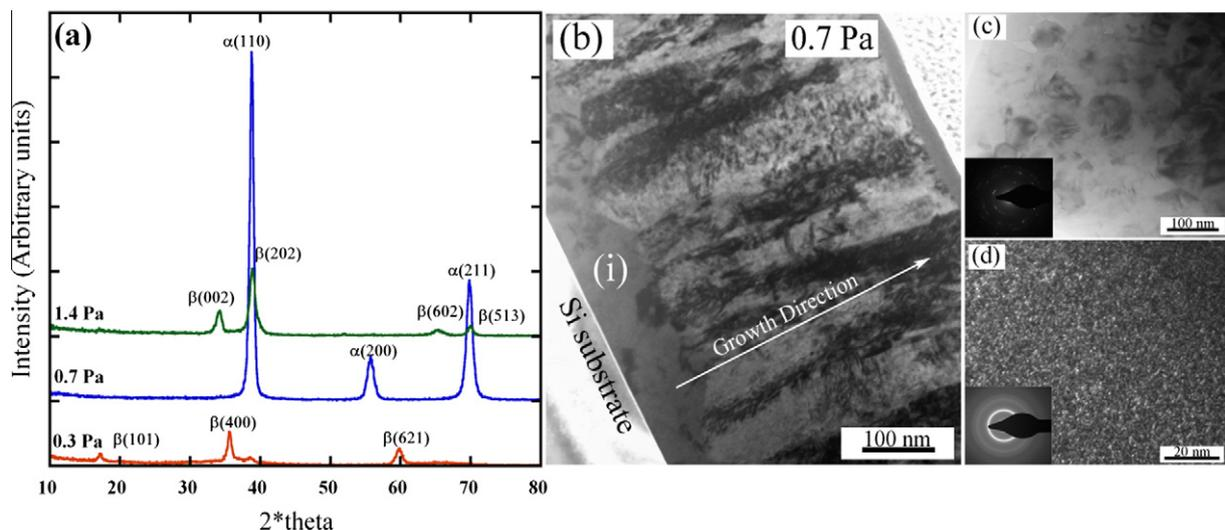
Figure 1. (a) Selected X-ray spectra of Ta films sputtered at a power of 100 W, with increasing sputtering pressures from 0.3 to 1.4 Pa. Notice the formation of  $\alpha$ -Ta at 0.7 Pa as shown by XRD and TEM in (b)–(d). (b) Cross-sectional image, arrow denotes growth direction. (c) Top-view image. (d) Plane-view image of the interface (i) layer showing the formation of ultra-small grains at the interface between film and substrate.
